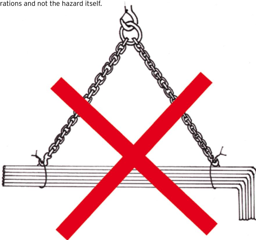
**DO NOT LIFT CUT AND BENT BUNDLES USING THE BUNDLE TIES THEY ARE NOT TESTED AS LIFTING EQUIPMENT AND ARE THEREFORE UNSAFE FOR LIFTING PURPOSES.
